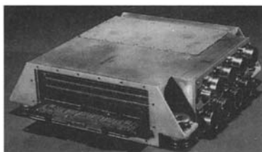
Fig. O.8 Full authority digital electronic control (FADEC).
