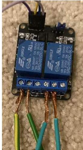
8. Connect In2 on the other side of the relay module to Digital 6 on the Arduino using a female-to-male connection wire
