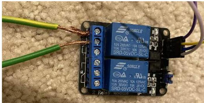
5. Connect 4 female-to-male wires to the other side of the relay board as seen.
