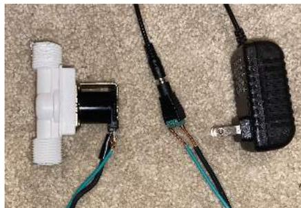
7. Take one of the cables (I chose the green one) and cut it through the middle, just like we did with the water boiler. Then connect the two new
