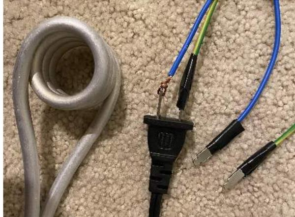
4. Then, find the middle of the green or blue wire (it doesn't matter which one) and cut it. Then cut a little piece of insulation to expose the wire itself. Plug in each end to the two left ports of K2 on the relay.
